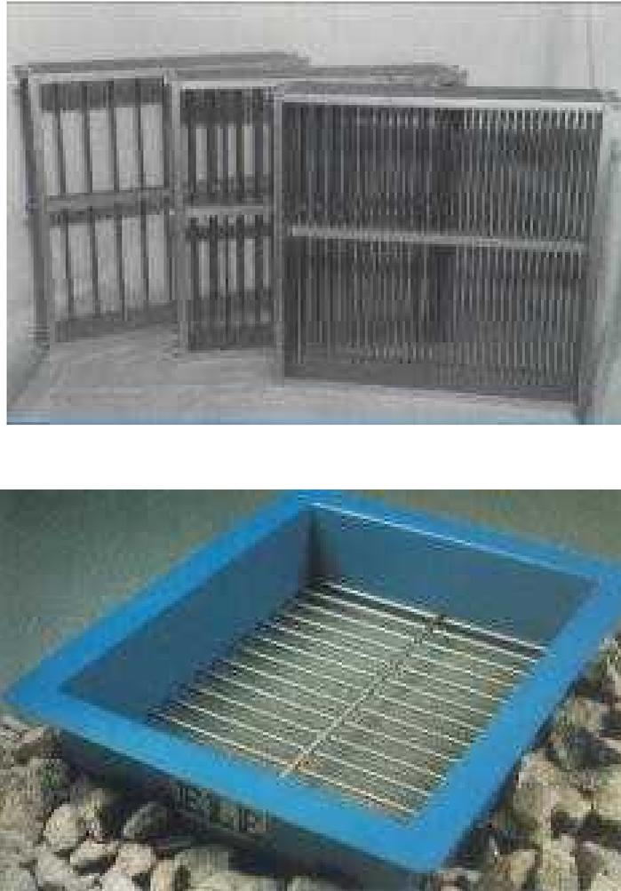
**Figure 3: Sieves used for the determination of flakiness index**
