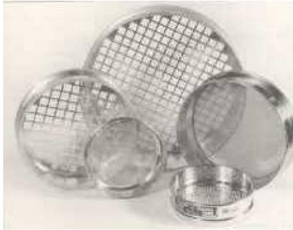
**Figure 2: Grading sieves**
